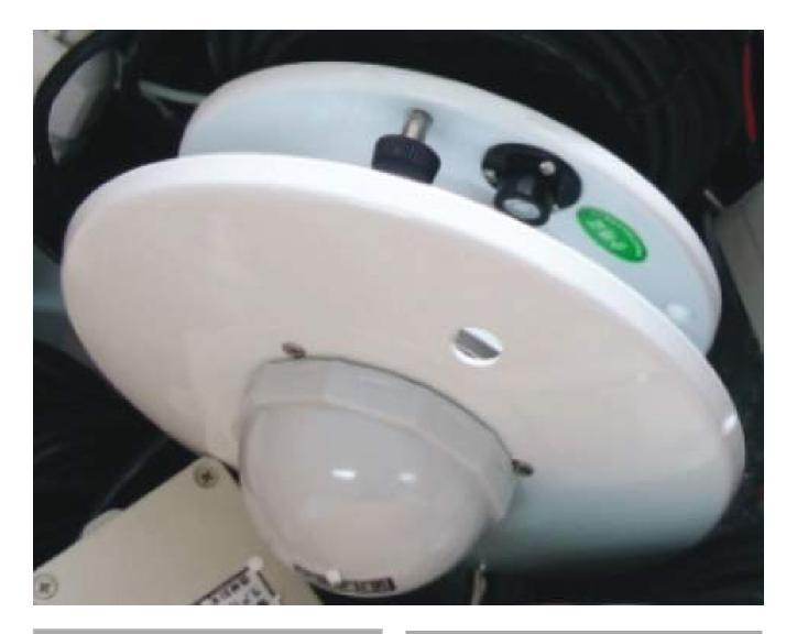
YDH-1 AWS Solar Radiation Sensor is an ISO-second-class pyranometer that monitors solar radiation for the full solar spectrum range. It connects directly to a YDH-1 RTU, and is used for many meteorological applications.
